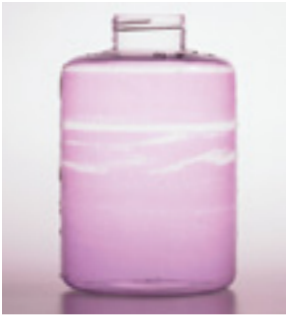
Figure 6. These clear bands were caused by debris in the medium scraping away cells as the bottle was rotated.
