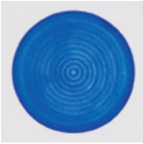
Figure 12. Vibration-induced concentric ring pattern in a 100 mm dish containing chick embryo fibroblasts that was stained 1 hour after plating.
