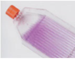
Figure 15. Vibration has caused the cells in this flask to attach in parallel rows. Moreover, the heavier cell density on the left side of this flask indicates the incubator shelf was not level.
