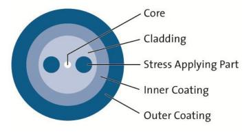
PANDA PM Specialty Optical Fiber design uses two stress applying parts to create an extremely high birefringence, resulting in fiber with excellent polarization maintaining properties. This design was invented and patented by Corning Incorporated. Corning continues to have a manufacturing partnership with Fujikura Ltd.
