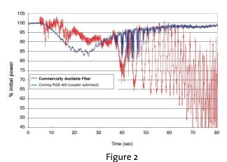
Single fiber taper loss pulls for RGB 400 and standard single-mode low wavelength fiber at 532 nm
