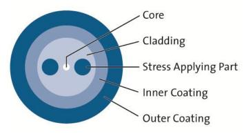
PANDA PM Specialty Optical Fiber design uses two stress applying parts to create an extremely high birefringence, resulting in fiber with excellent polarization maintaining properties. This design was invented and patented by Corning Incorporated. Corning continues to have a manufacturing partnership with Fujikura Ltd.
