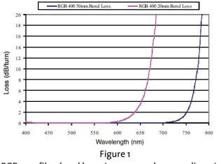
RGB 400 fiber bend loss at 20 mm and 50 mm diameters
