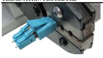
**Step 15** Crimp the Crimping Tube by the LC Slimpac3 crimping tool. The hexagonal die dimension is 4.52mm.
