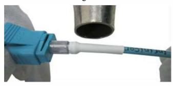
**Step 16** Use heating gun to heat the shrinking tube.
