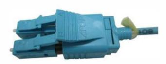
Step 13 Then the back housing inserted where is 45 ° from the local to the Back Housing push and close together with the Lower Housing.
