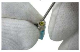
**Step 3** Have the epoxy ready according to the manufactures instructions and put part of the mixed epoxy into a small container. The rest of epoxy should be stored in the freezer for latter use.
