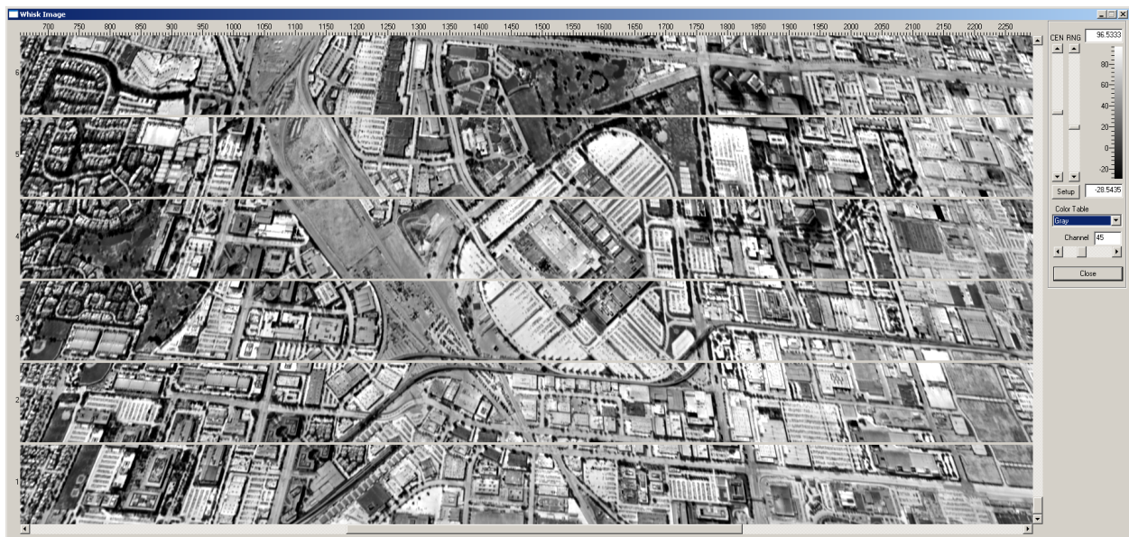
Figure 3. Screen shot showing the center two-thirds of 6 whisks excerpted from a 100-whisk Mako dataset acquired over an urban area in Los Angeles. The aircraft flight path is from bottom to top of this view, roughly along the center, and the Mako gimbal mirror slews to the left and right of nadir. Each whisk consists of 128 vertical pixels. In this dataset each whisk contains 2800 frames of data (horizontal pixels, corresponding to slightly more than \pm 40^\circ around nadir), for a total of 358,400 pixels per whisk. Each pixel has a 128-channel spectrum associated with it. This data was acquired at 12,500 ft. AGL, at which altitude the pixel size is \sim 2 meters. The picture also clearly shows the overlap between whisks, which is a programmable quantity with a default value of 10%.
