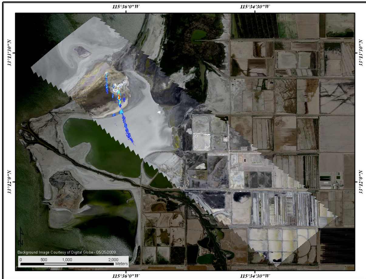
Figure 6. Ammonia plumes (colored lineaments in the upper left quadrant of the image, the longest of which is ~1.5 km in length) at the SE margin of the Salton Sea, as detected with the Mako sensor. The plumes are superimposed on the false color thermal radiance map (using Mako spectral channels at R=11.72, G=10.27, B=8.81 microns). White areas represent hot regions and signify geothermal activity at the surface. These data were acquired from an altitude of 6700 ft. AGL. (Background visible image courtesy of DigitalGlobe.)
