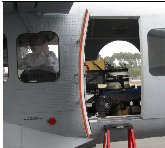
Figure 2. Mako sensor installed in the rear of a Twin Otter aircraft, where it looks down through a rectangular port in the bottom of the fuselage.
