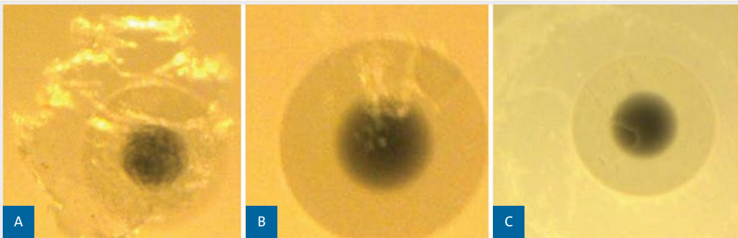
Figure 5: Particles deliberately placed over fibers in LC connectors to study effect of occlusion on IL: (a) Delrin®, (b) Ultem®, (c) skin flake.
