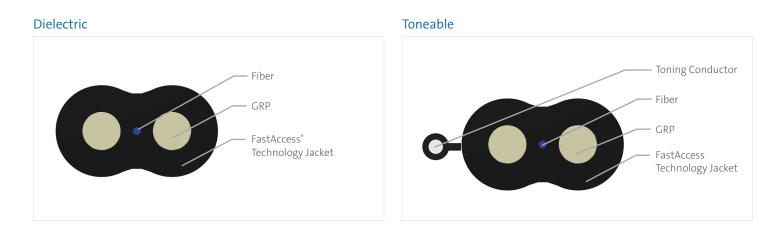
As an industry leader in optical connectivity products, Corning designs and manufactures the ROC<sup>®</sup> drop cable assembly with factory-terminated, environmentally sealed and hardened connectors to reduce the cost and time of drop cable deployment. Corning hardened connectors provide superior durability and reliability in the drop segment of the network. This assembly also offers significant improvements in cable management.
