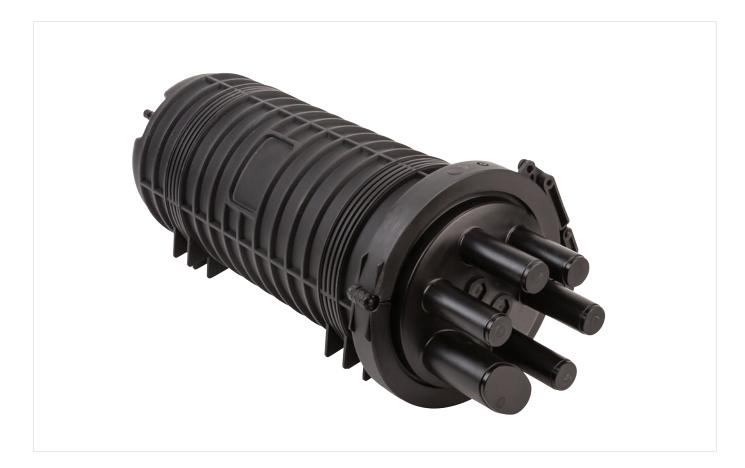
Fiber Optic Splice Closure 2179 CD accommodates various splice applications, such as express, branch, or drop. Using mechanical sealing technology, the dome seals from base to dome – preventing ingress and enabling easy re-entry. Plus, the cable ports are designed for use with heat-shrink sealing technology for robust protection from the elements.
